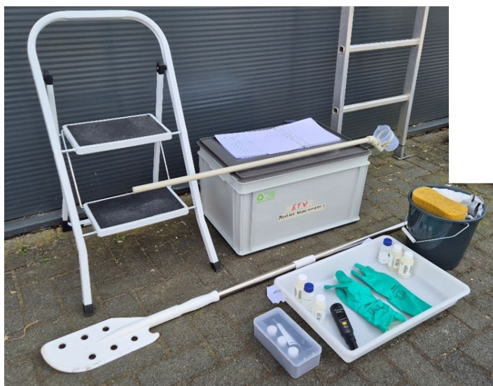
Figuur 1.1 Meetset watermonsters dompelcontainer
