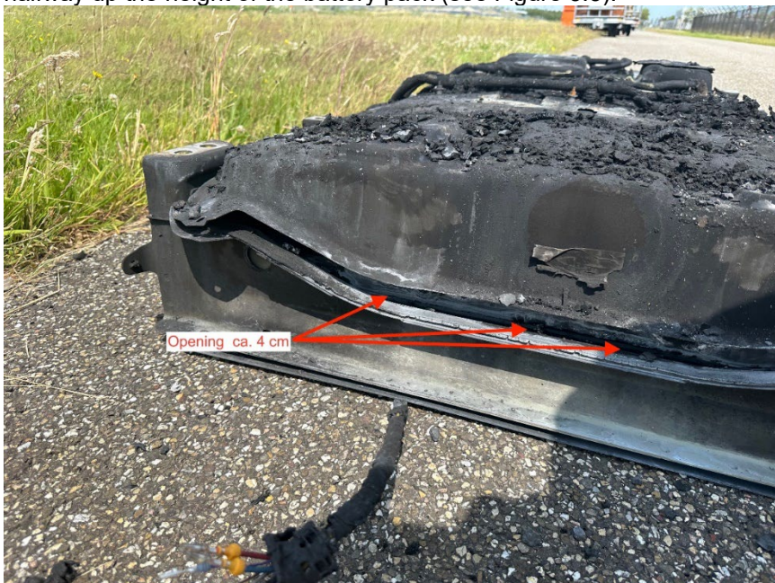
Figure 5.5 Opening of battery pack by overpressure
