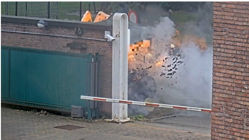
Figure 2.3 Explosive ignition of a vapour cloud (photo: unknown)
