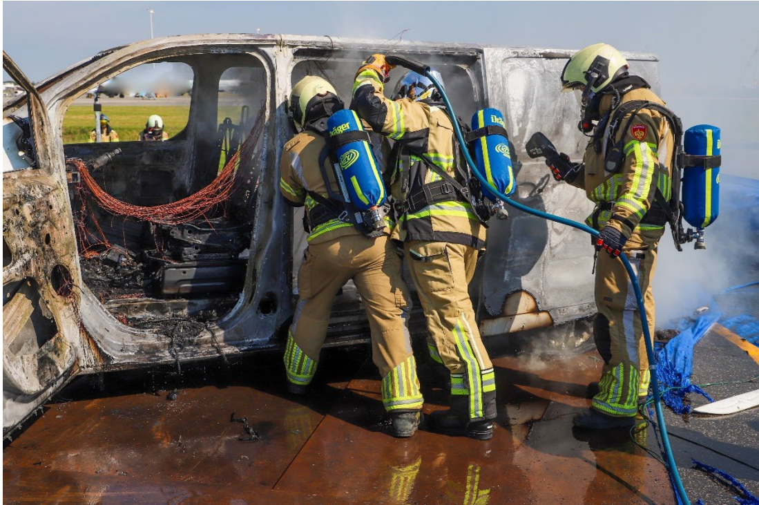
Figure 5.1 Locating and monitoring hot spot and preparing for penetration
