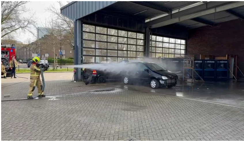
Figure 4.5 Deployment of UHP extinguishing system to bust the windows (photo: Haaglanden Safety Region)
