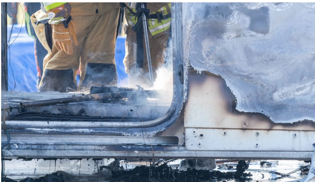
Figure 5.2 Steam formation during deployment of UHP extinguishing system
