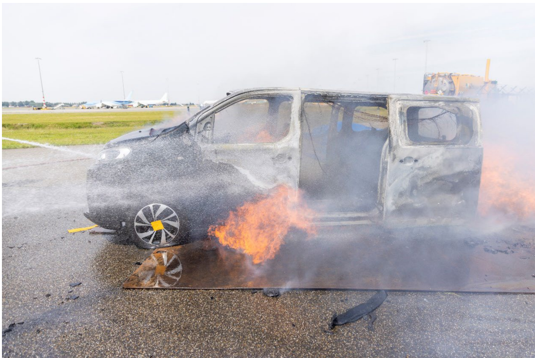
Figure 5.7 Jet fire from battery pack (under the front passenger door)
