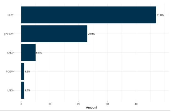
Figure 4.1 Fires (%) broken down by vehicle technology / fuel types of the AFVs
