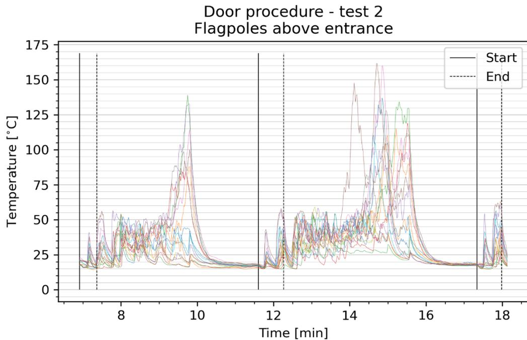
Figure 2.33 Temperature development above the front door during door procedure 2
