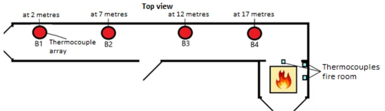
**Figure 1.8 Floor plan (view from above) with locations of measuring equipment**
