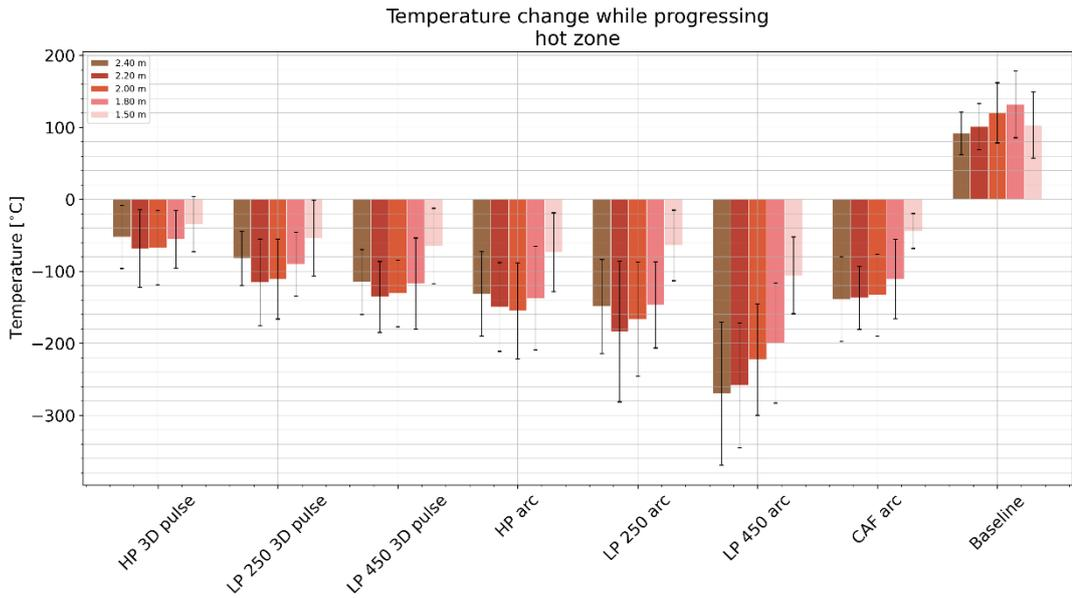
Figure 2.2 Changes in temperature for each fire extinguishing system and attack method in the hot zone, grouped by attack method
