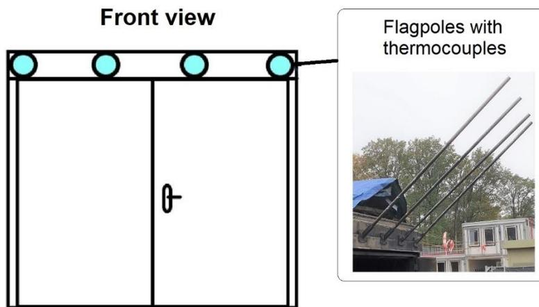
**Figure 1.9** Front view of building with locations of measuring equipment
