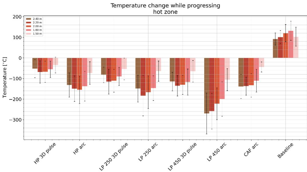
Figure 2.3 Changes in temperature for each fire extinguishing system and attack method in the hot zone, grouped by extinguishing system
