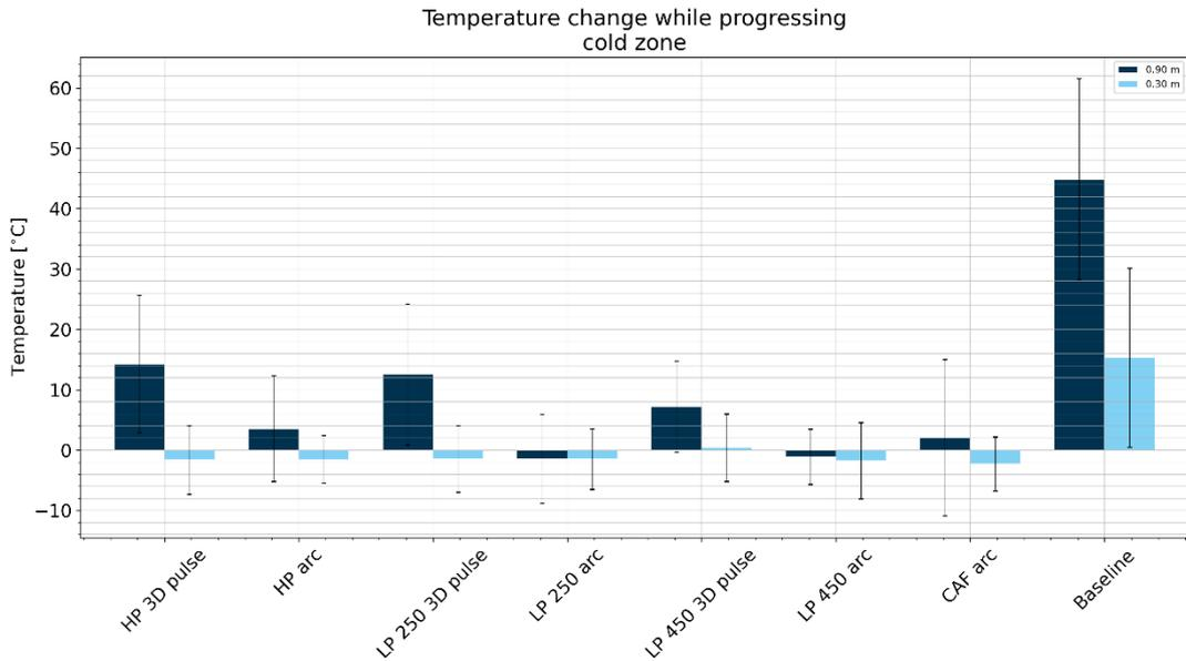
**Figure 2.6** Changes in temperature for each fire extinguishing system and attack method in the cold zone, grouped by extinguishing system
