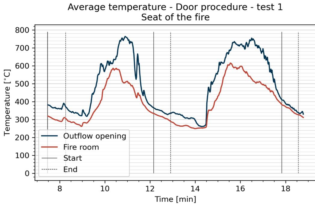
Figure 2.34 Temperature in the fire room during door procedure 1
