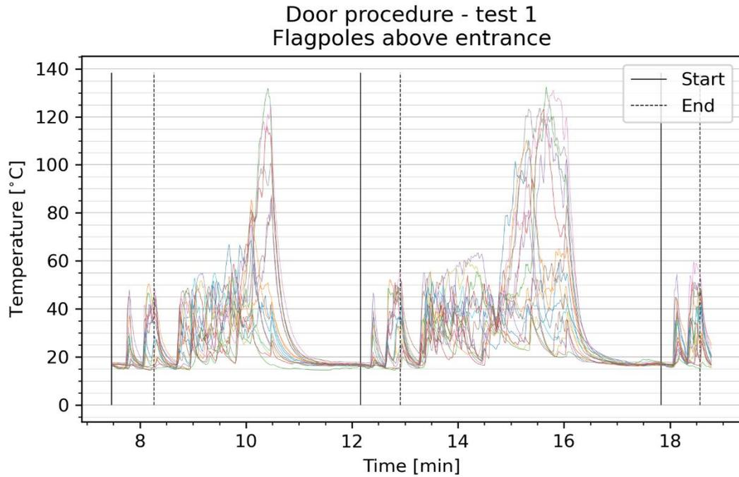
Figure 2.32 Temperature development above the front door during door procedure 1
