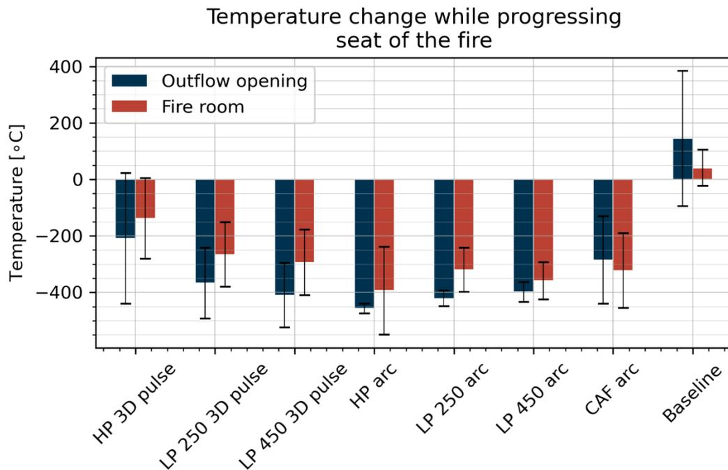
Figure 2.19 Changes in temperature in the fire room for the individual fire extinguishing systems and attack methods while progressing
