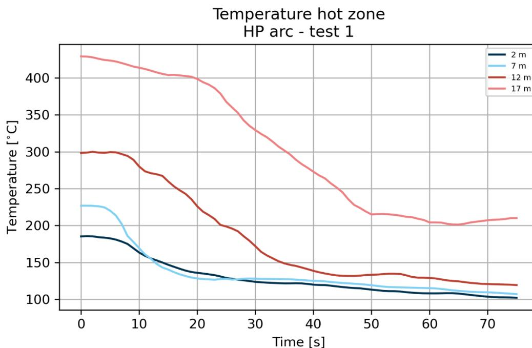
**Figure 2.16** Temperatures in the hot zone while progressing at different distances in the corridor
