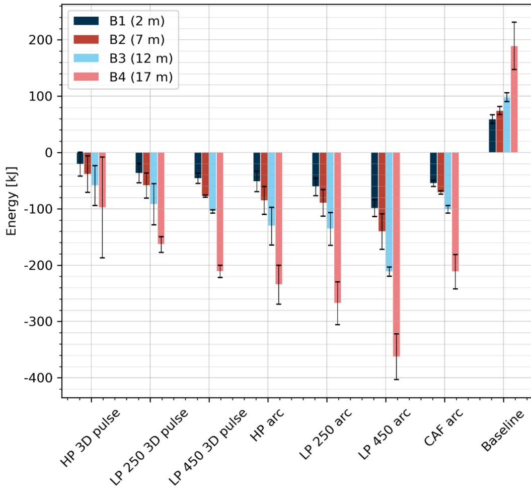
Figure 2.8 Changes in energy for each fire extinguishing system and attack method in the hot zone, grouped by attack method
