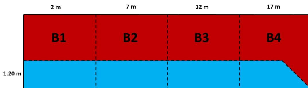
**Figure 1.16 Side view of division of the corridor into vertical segments and horizontal hot (red) and cold zones (blue)**
