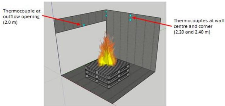
Figure 2.148 Diagram of the design of the seat of the fire in the fire room
