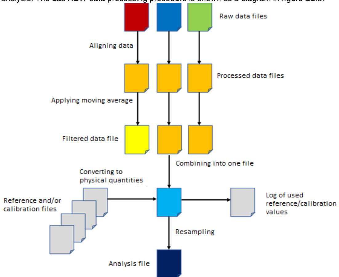
Figure B2.3 Diagram of the processing of LabVIEW data
