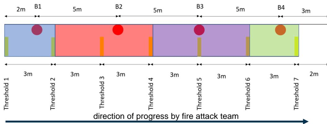
**Figure 18: Distribution of measurements for calculating the fire attack team's exposure to radiation**
