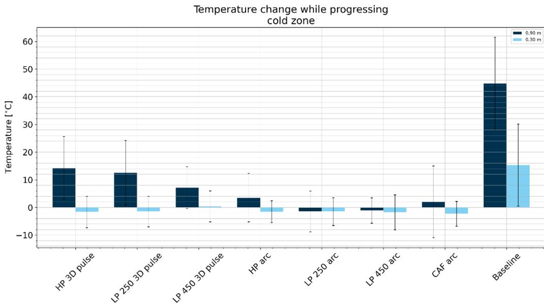
Figure 2.5 Changes in temperature for each fire extinguishing system and attack method in the cold zone, grouped by attack method
