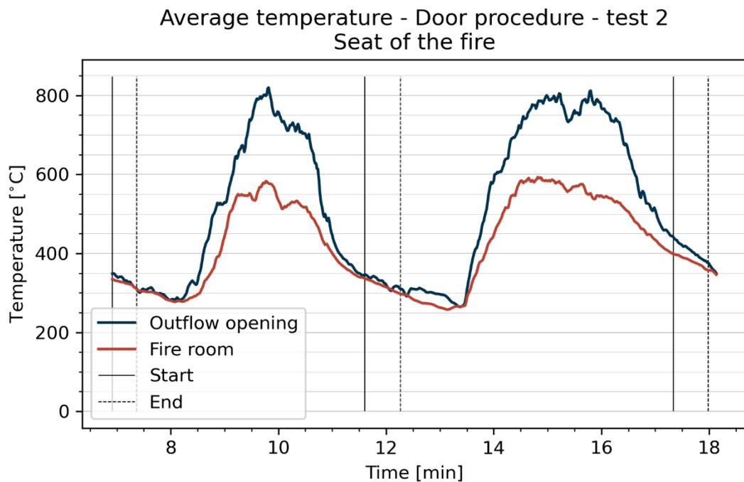
Figure 2.35 Temperature in the fire room during door procedure 2
