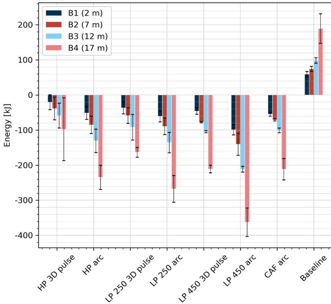
Figure 2.9 Changes in energy for each fire extinguishing system and attack method in the hot zone, grouped by extinguishing system
