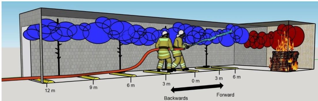
**Figure 2.15** Smoke gas in front of and behind the fire attack team with an HP attack with the arc method
