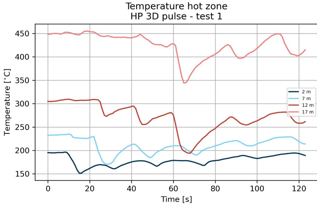
**Figure 2.14** Temperatures in the hot zone while progressing at different distances in the corridor
