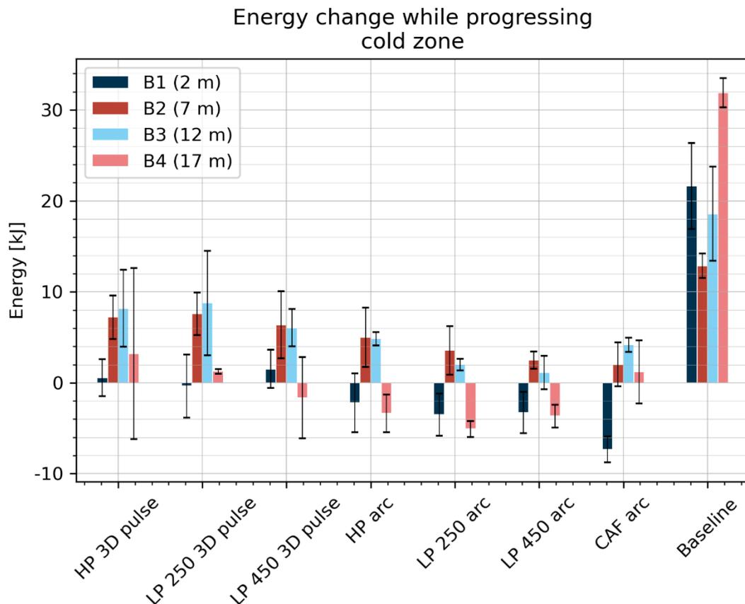
Figure 2.11 Change in energy in the cold zone while progressing for each fire extinguishing system and attack method, grouped by attack method
