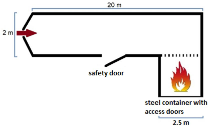
Figure 1.1 Floor plan of the test location
