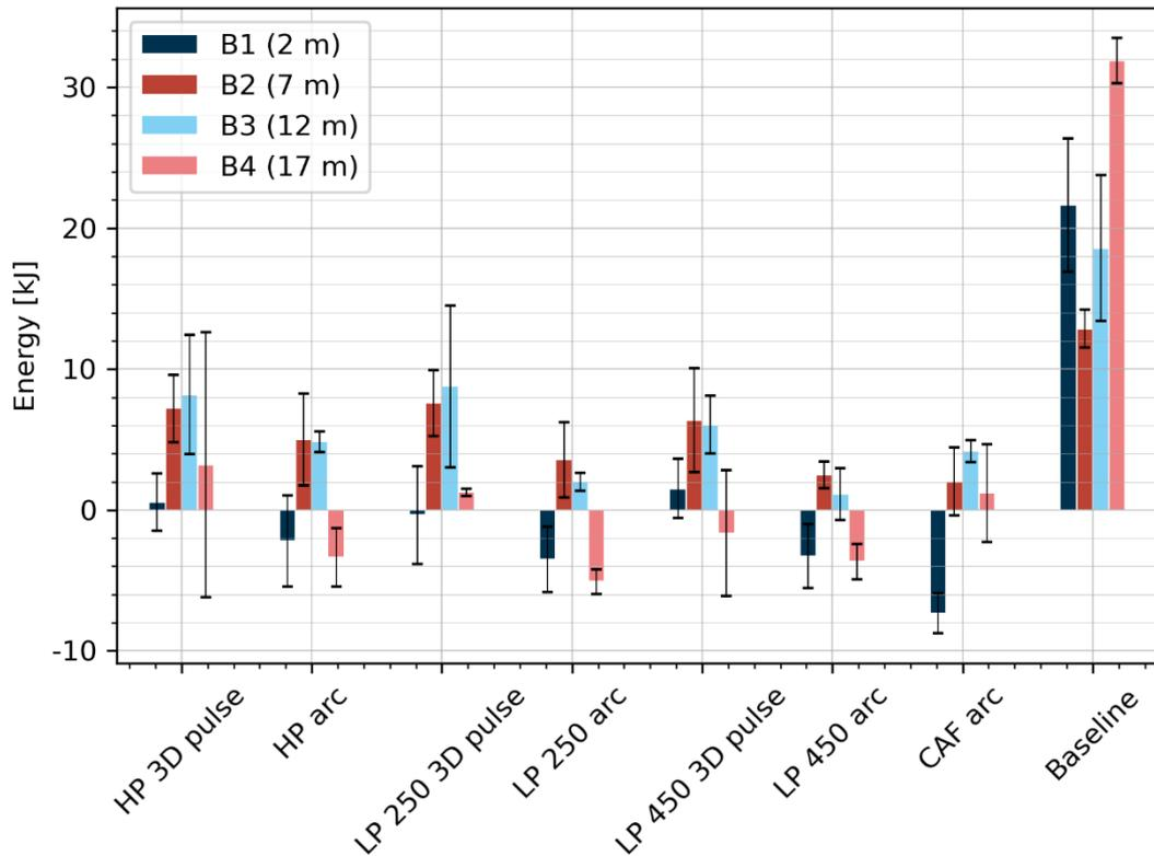
Figure 2.12 Change in energy in the cold zone while progressing for each fire extinguishing system and attack method, grouped by fire extinguishing system
