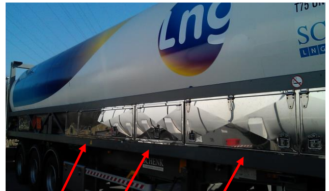
LNG tanker truck, with control box on the side
