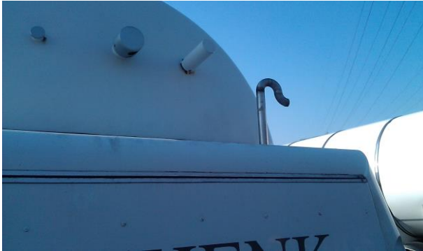
Tanker truck blow-off valve
