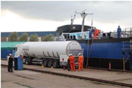
Mobile bunker location from tanker truck
