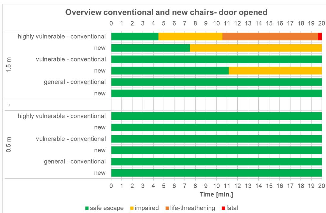
**Figure 2.53 Times for the possibility of escape and survivability of the tests with the door open**
