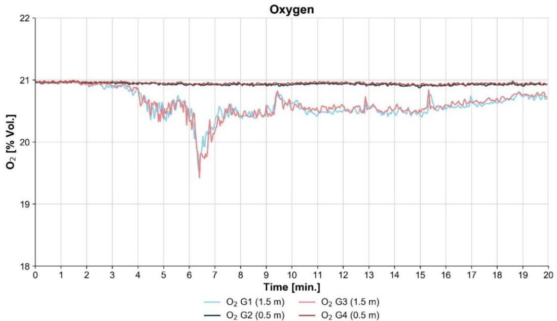
Figure 2.41 Oxygen concentration at 4 locations [% vol.] for test 4
