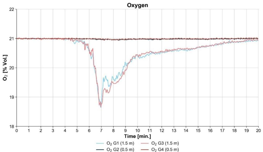
Figure 2.23 Oxygen concentration at 4 locations [% vol.] for test 2
