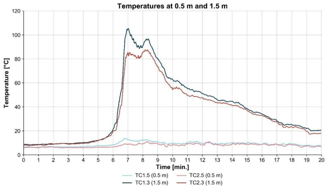
Figure 2.21 Temperatures at 0.5 and 1.5 m height [°C] for test 2
