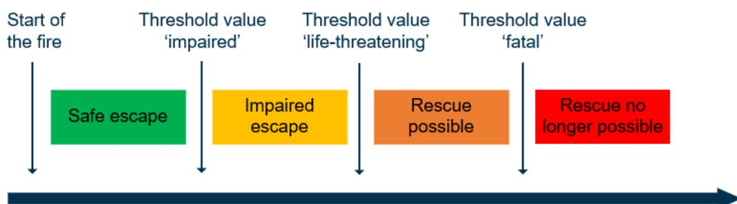
Figure 1.6 Diagram of the possibility of escape and survivability in the event of fire
