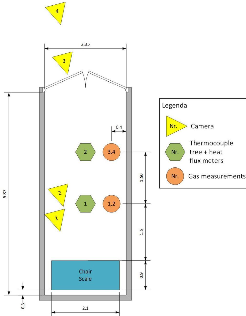
Figure 1.3 Floor plan with measurement devices
