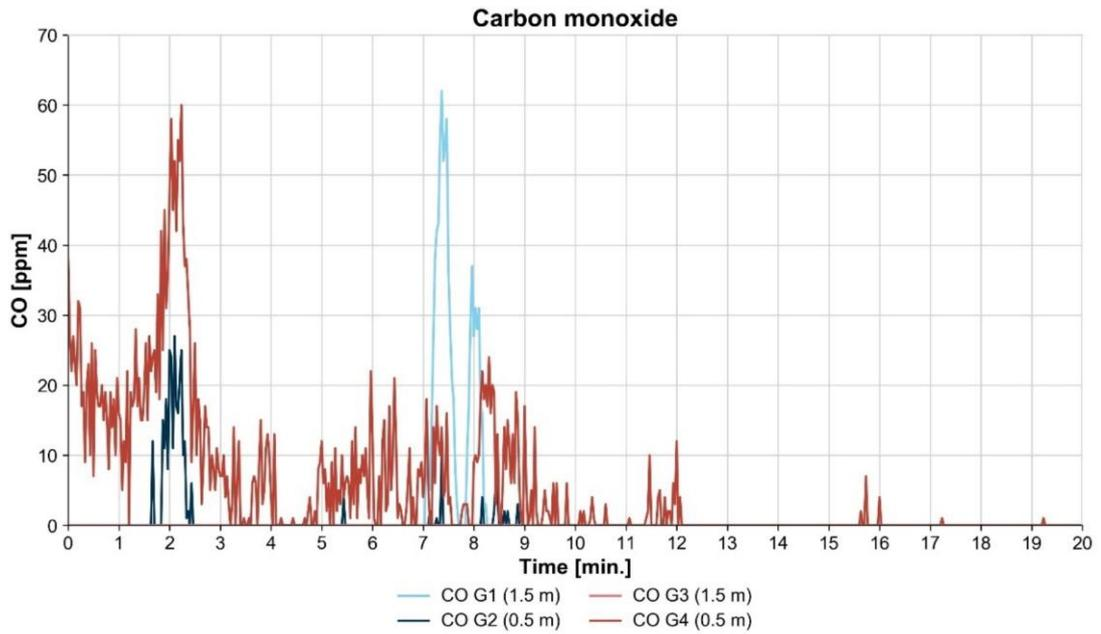
Figure 2.22 Carbon monoxide concentration at 4 locations [ppm] for test 2
