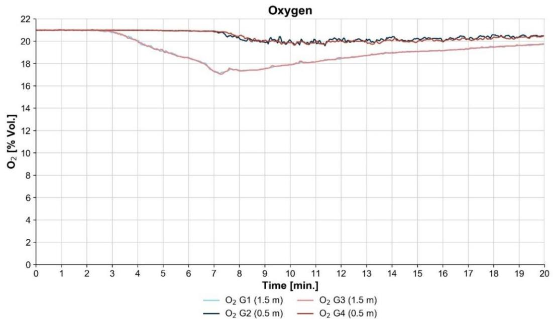
Figure 2.32 Oxygen concentration at 4 locations [% vol.] for test 3
