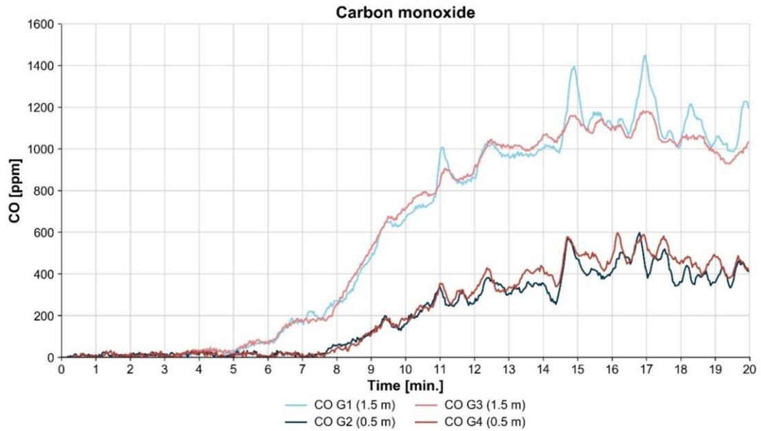
Figure 2.31 Carbon monoxide concentration at 4 locations [ppm] for test 3
