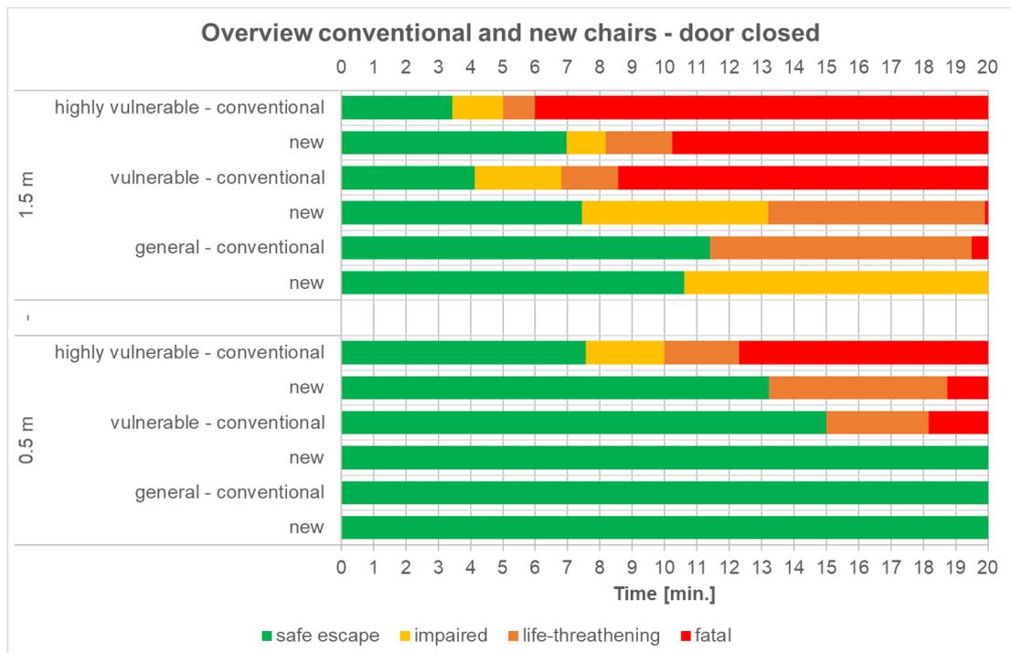
Figure 2.52 Times for the possibility of escape and survivability of the tests with the door closed
