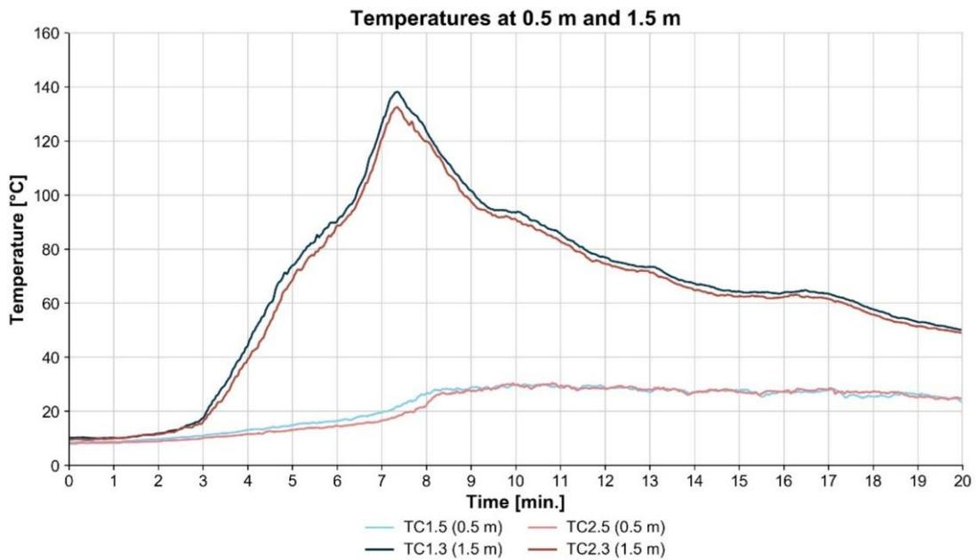
Figure 2.30 Temperatures at 0.5 and 1.5 m height [°C] for test 3
