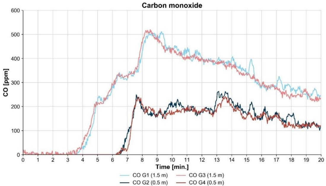
Figure 2.13 Carbon monoxide concentration at 4 locations [ppm] for test 1
