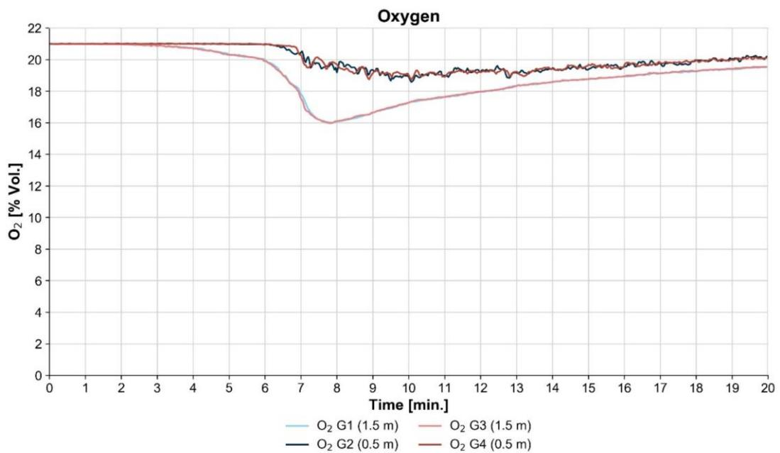
Figure 2.14 Oxygen concentration at 4 locations [% vol.] for test 1
