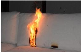
Figure 24: Start open flame test
