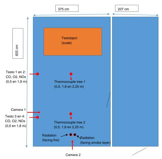
Figure 7: Measurement tools and location on the floor plan
