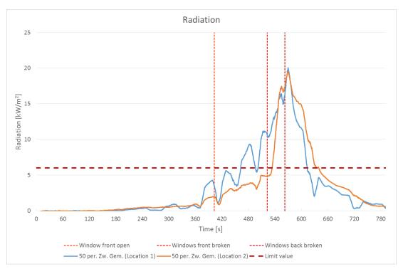
Figure 29: Radiation heat flux graph
