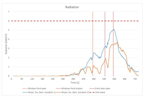
Figure 42: Radiation heat flux graph
