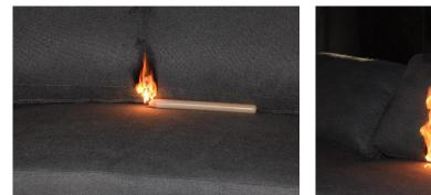
Figure 11: Start open flame test
