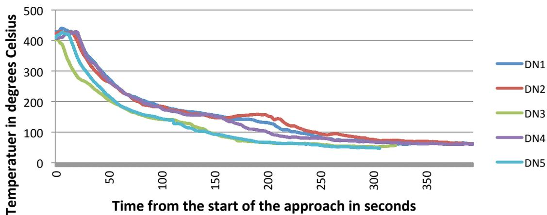
Figure 16: variation in temperature distributor nozzle tests
