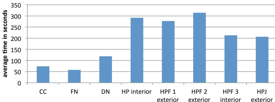
Figure 8: smoke gas layer < 150°C for the various systems
