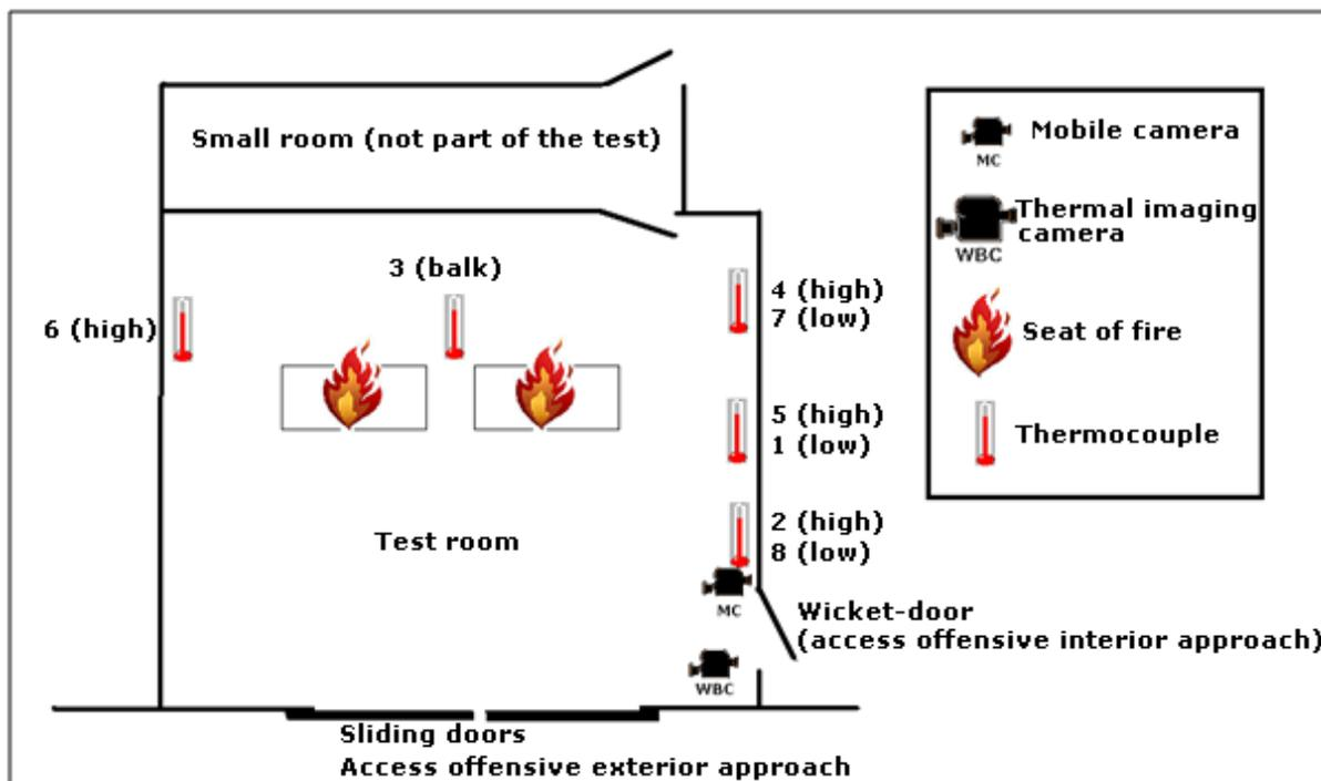
Figure 5: Schematic drawing of the test area
