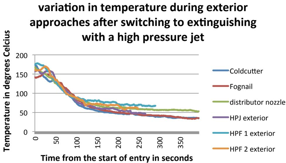
Figure 13: average temperature upon entering per exterior approach
