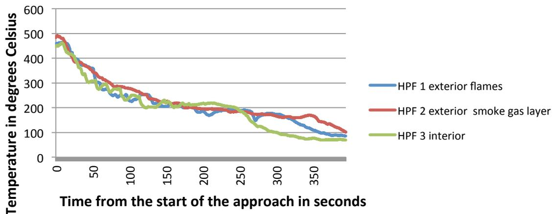
Figure 19: variation in temperature high pressure foam tests
