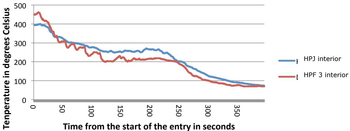
Figure 18: average temperature upon entering in interior approaches
