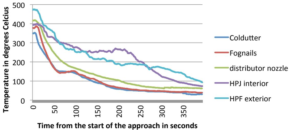
Figure 6: average temperature smoke gas layer TC-6
