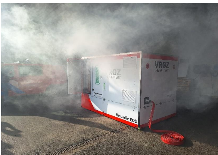
Figure 2.6 Mobile ESS mock-up used for fire fighter training (picture: Tom Hessels)
