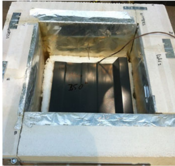
Figure 3. A sample in the furnace during the mass-loss experiment while exposed to the heat from below. [Colour figure can be viewed at wileyonlinelibrary.com ]
