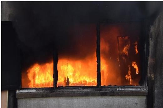
Figure 26: Fully developed fire
