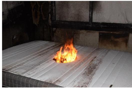
Figure 38: Fire spread over mattress
