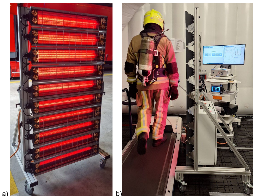
Figure 1.1 Radiation panel (a); and an exercising person at the side of the panel (b)
