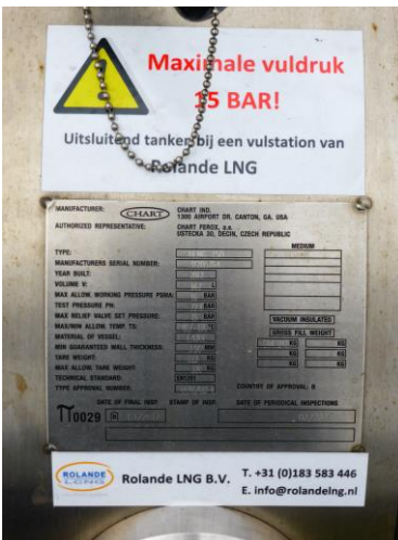
Specifications of the LNG tank and contact details of the operator are on the fuel tank.
