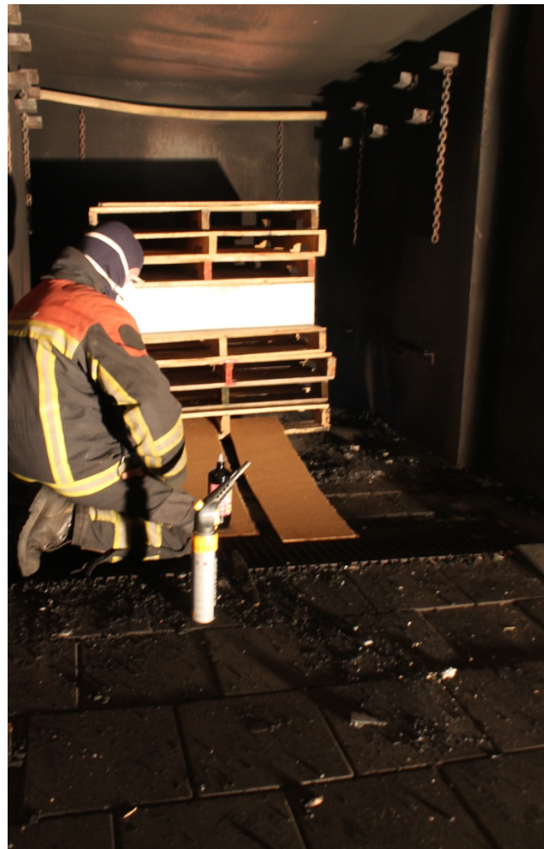
Illustration 3.2: Composition and ignition of the fire load
