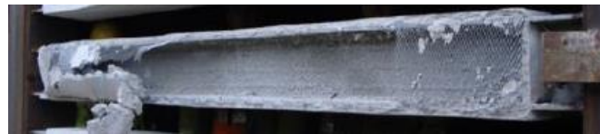
Figure 37 - Boxed PFP construction after an explosion test
