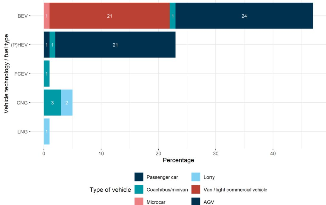
Figure 4.3 Fires broken down by type of vehicle broken down by vehicle technology / fuel types.
