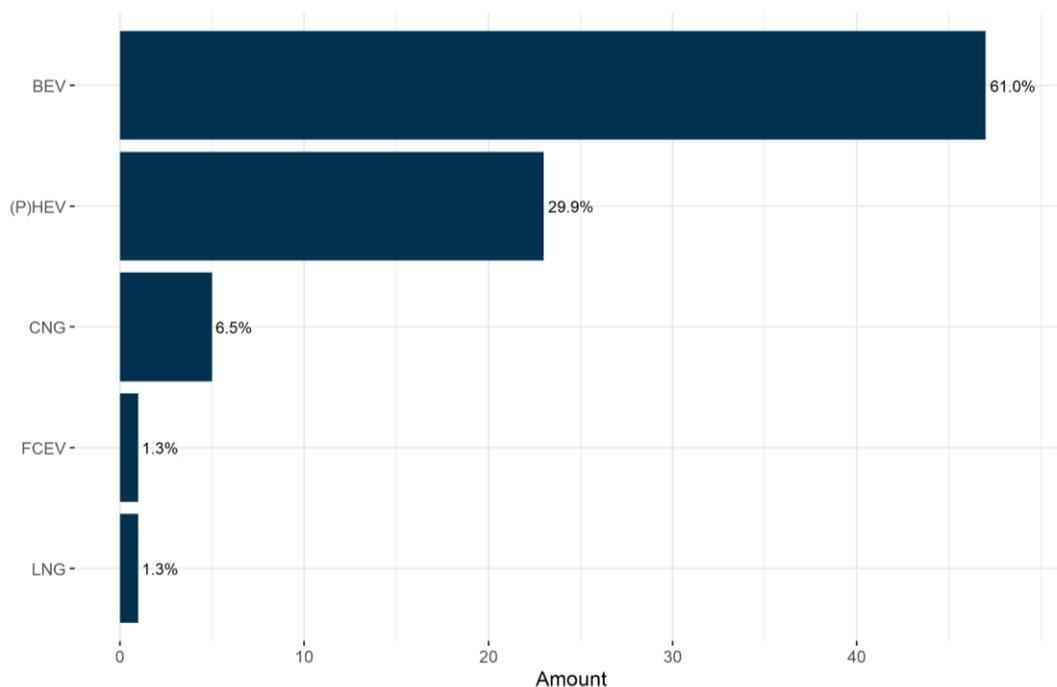
Figure 4.1 Fires (%) broken down by vehicle technology / fuel types of the AFVs
