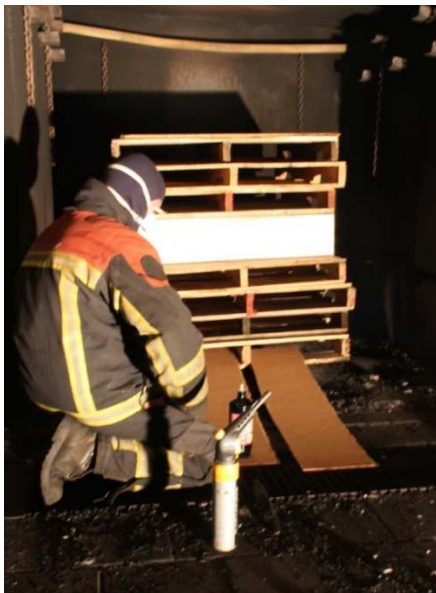
Figure 2.3. Composition and ignition of the fire load
